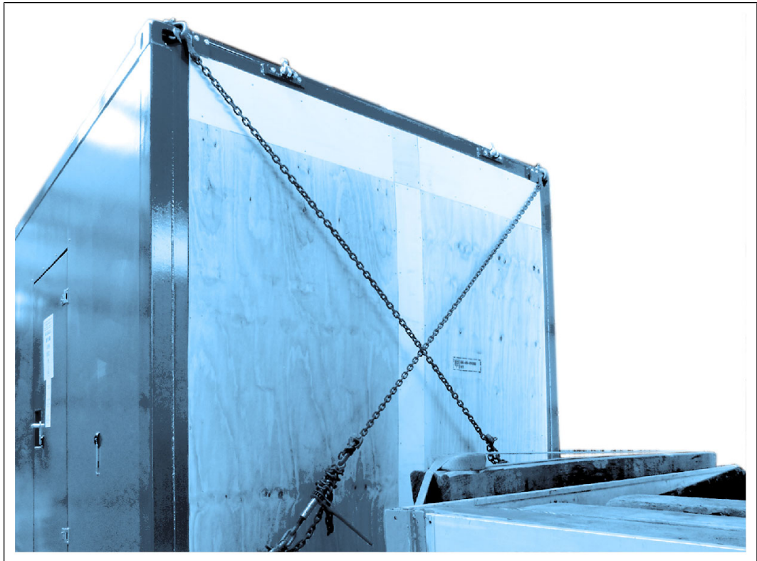
4262384267: Fixing a container for transport on a low loader
